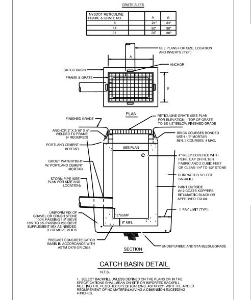
2. IF CLEAN STONE BEDDING IS USED THE BEDDING SHALL BE ENCIRCLED WITH FILTER FABRIC TO PREVENT SOILS FROM ENTERING THE VOIDS OF THE STONE
